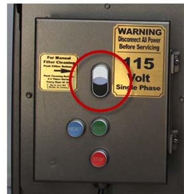
The filters will clean better with the machine turned off.
